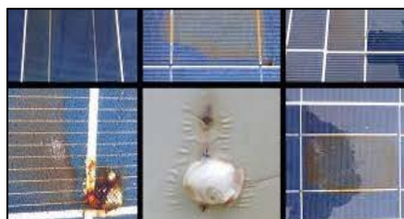
Figure 2 : Different types of hotspots in a PV panel.
